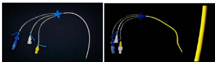
Figure 1: Uncoated catheter and Catheter coated with top coat of drug & PVP, base coat of drug and PU.
